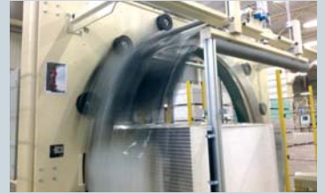
Automatic spiral wrapping machine in production line for Gypsum wallboard
