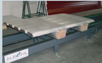
Stretch film packaging with automatic wood/EPS runners feeder. No steel strap required.
