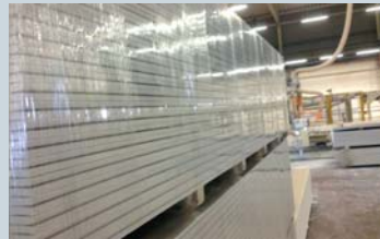
Stretch film packaging with automatic wood/EPS runners feeder. No steel strap required.
